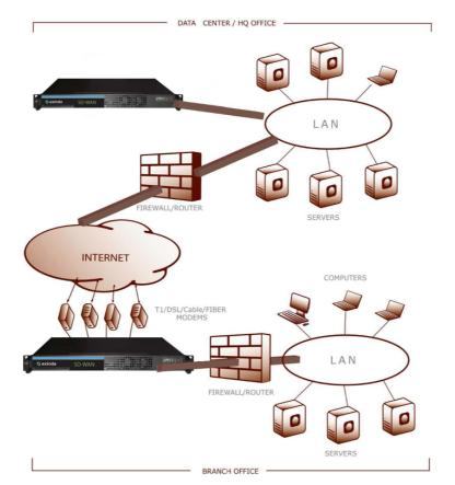
The two Exinda devices form a transparent, high-speed data tunnel between them by combining access resources on each side.
