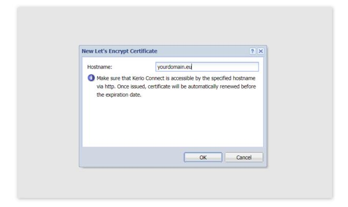
Opening port 80 might be seen as a security risk for the server and users. It is therefore recommended to only use an encrypted connection with Kerio Connect. It will force users to use webmail over port 443 / HTTS instead of an unsecured HTTP.
